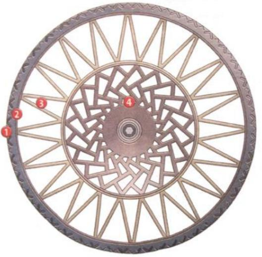
Cable-reinforced band of conventional "tyre" rubber with molded tread
